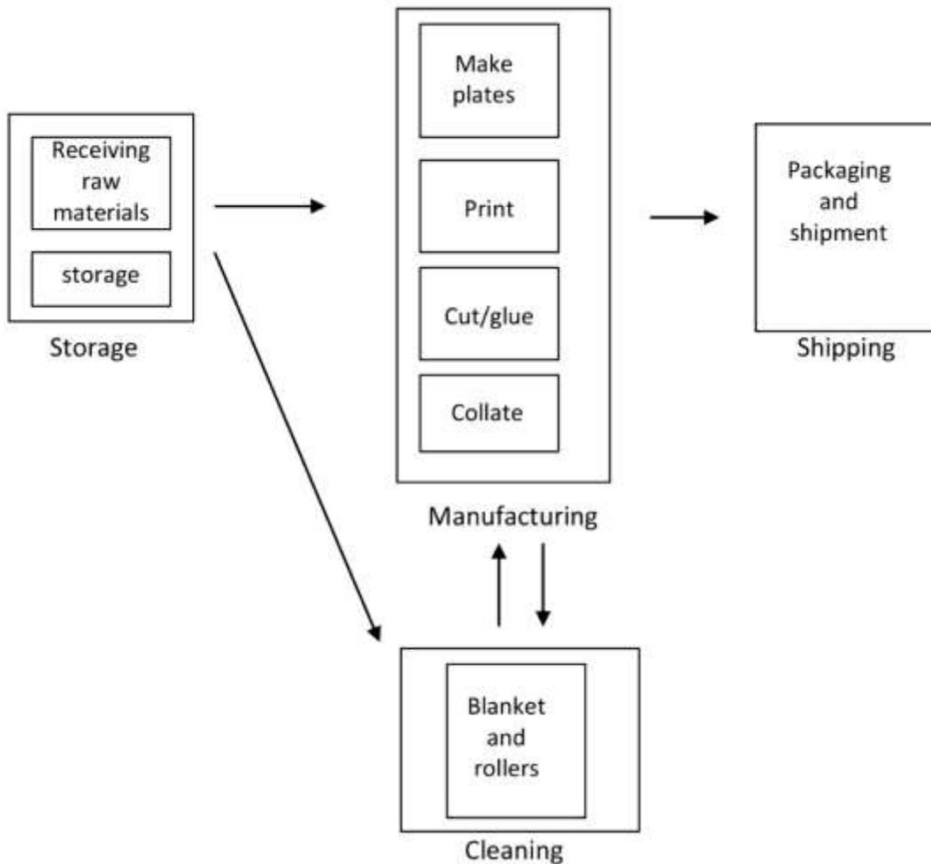
A tour of the facility was undertaken to identify individual processes. These processes were broken down into the storage, manufacturing, cleaning and shipping stage.
