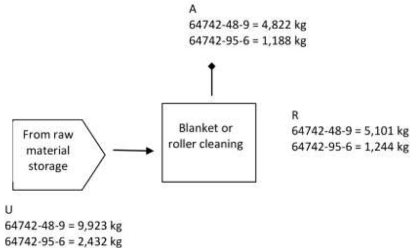
VOC is used as a manual and automatic cleaner for blankets and rollers. When cleaning the rollers, the drip tray is lined with wipers, solvent is dispensed onto the top roller and dirty solvent collects in the drip tray. The saturated wipers are shipped off site for laundering.
